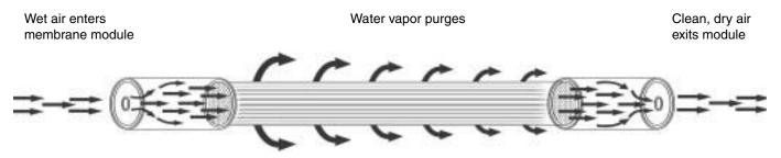
Water vapor permeates through hollow membrane fibers
